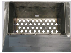
Brazier is cleaned well, with all holes visible
