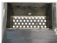
Brazier well cleaned, with all holes visible
