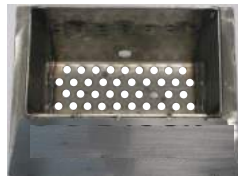
Brazier well cleaned, with all holes visible
