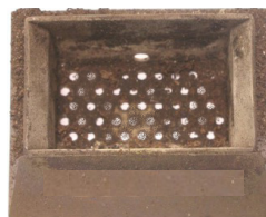
Brazier requiring cleaning having its holes blocked by the ashes
